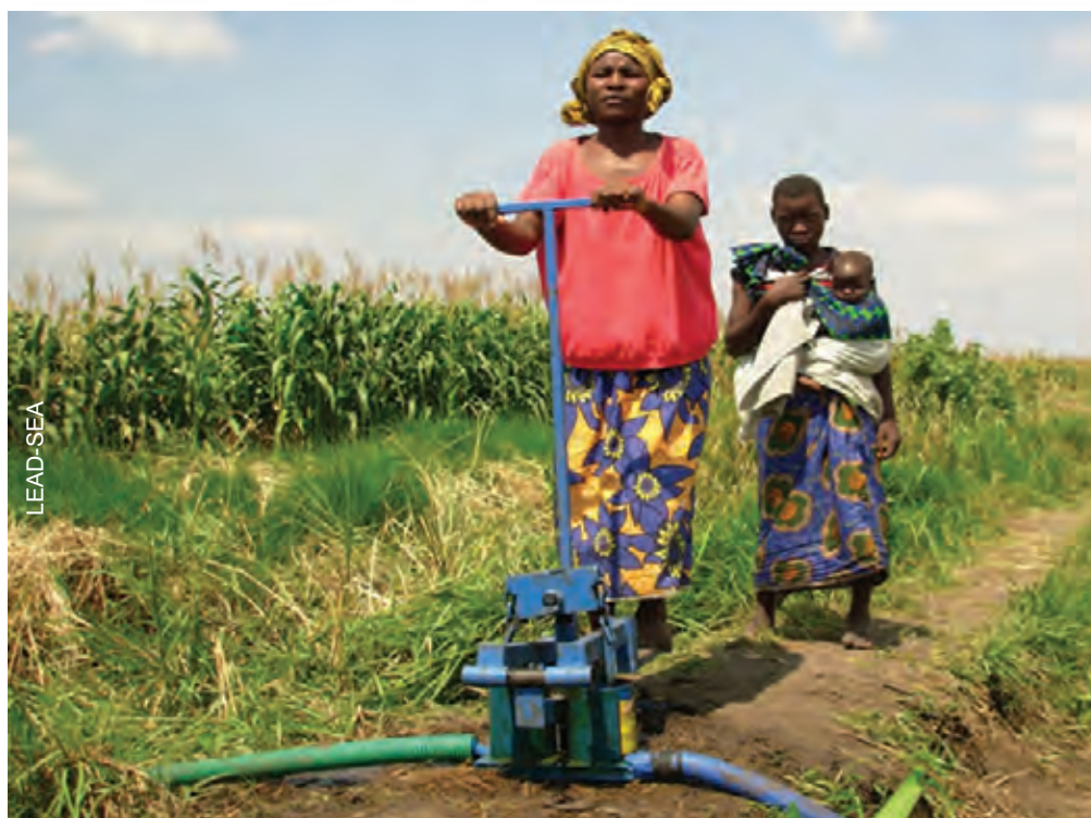
Treadle pump for irrigation
