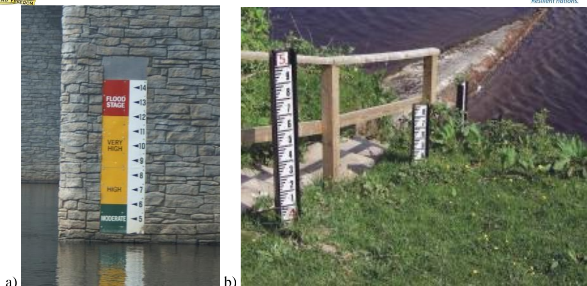
Fi 13: Examples of Staff Gauges- (a) Colour coded gauge, (b) sequential gauge set in river bank (NIRAS Report on CBEWS 2018)
